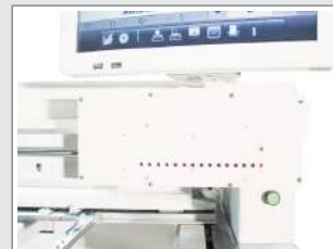
Color change box • By applying a ball screw, the color change speed is increased and accurate positioning is enabled.
